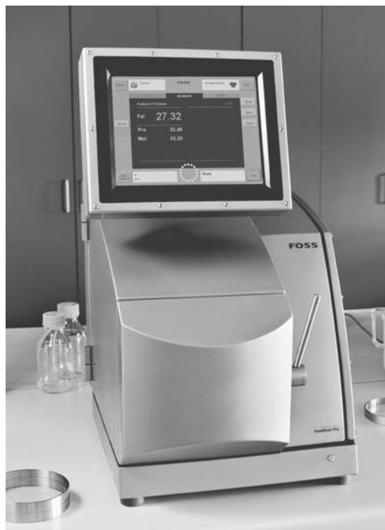
Fig. 5.7 Foss FoodScan™ Pro NIR analyser with IP65 waterproof cabinet for analysis of butter and other solid and semi-solid food products. With permission of Foss UK.
