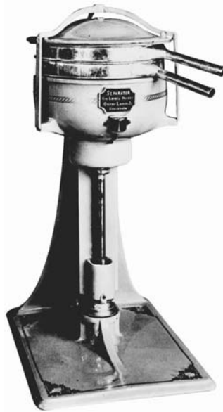
Fig. 3.4 A view of one of the first separators the Alfa 1 made in 1882. Reproduced with permission of Tetra Pak AB, Lund, Sweden.
