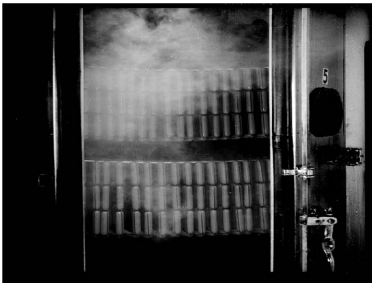
Fig. 10.6 Atomization cloud in a smokehouse (courtesy of Red Arrow Products Company LLC, Manitowoc, Wisconsin, USA).
