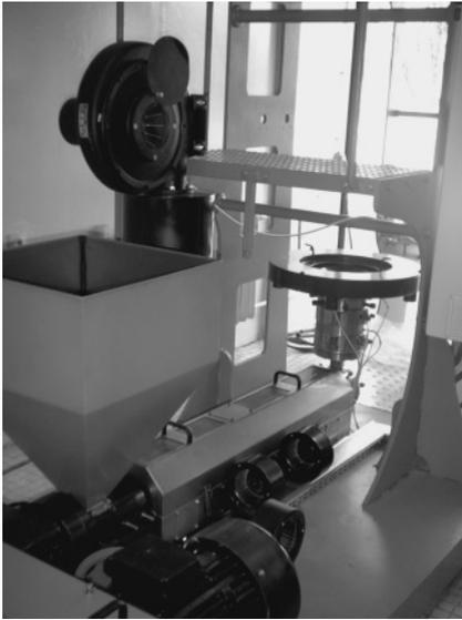
Figure 9.1 Stand for film extrusion processing.
