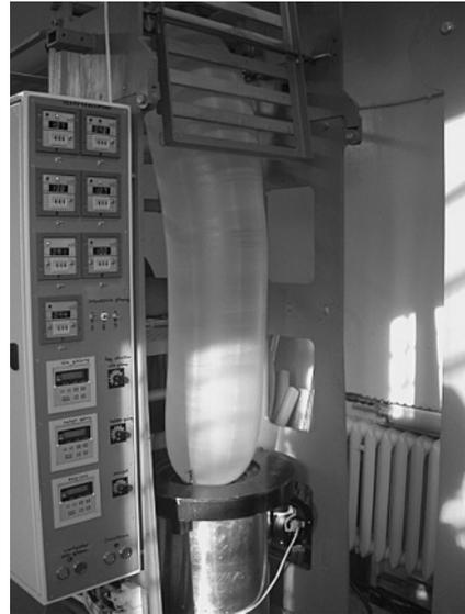
Figure 9.2 TPS film-blowing.
