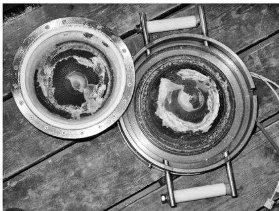
**Figure 5.2** Starch/glycerol mixtures a) before and b) after shearing–heating process in shear cell device.
