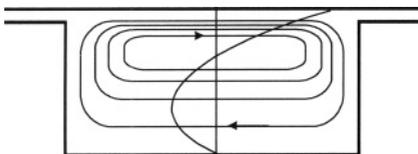
Figure 6.4 Rotating flow in the cross-channel direction.
