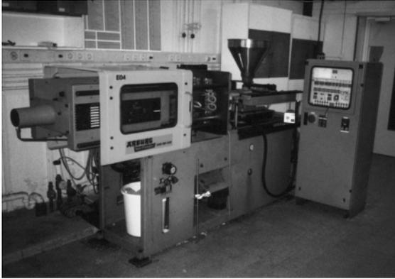
Figure 10.1 Injection-molding machine (ARBURG 220H90-350).
