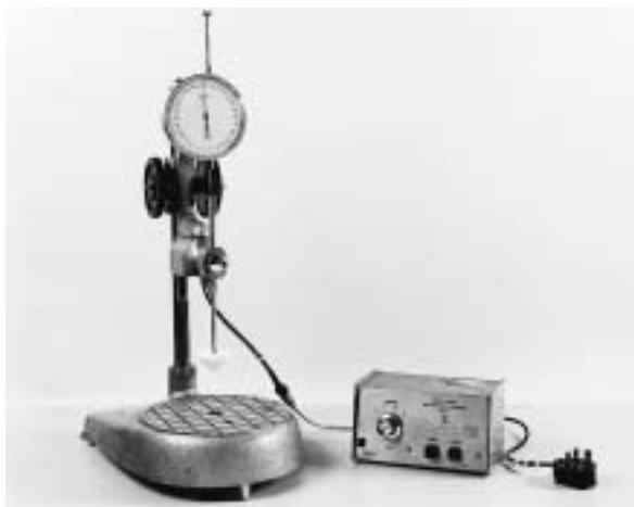
Fig. 10.3 Standard penetrometer of the type that can be employed to measure the consistency of set yoghurt
