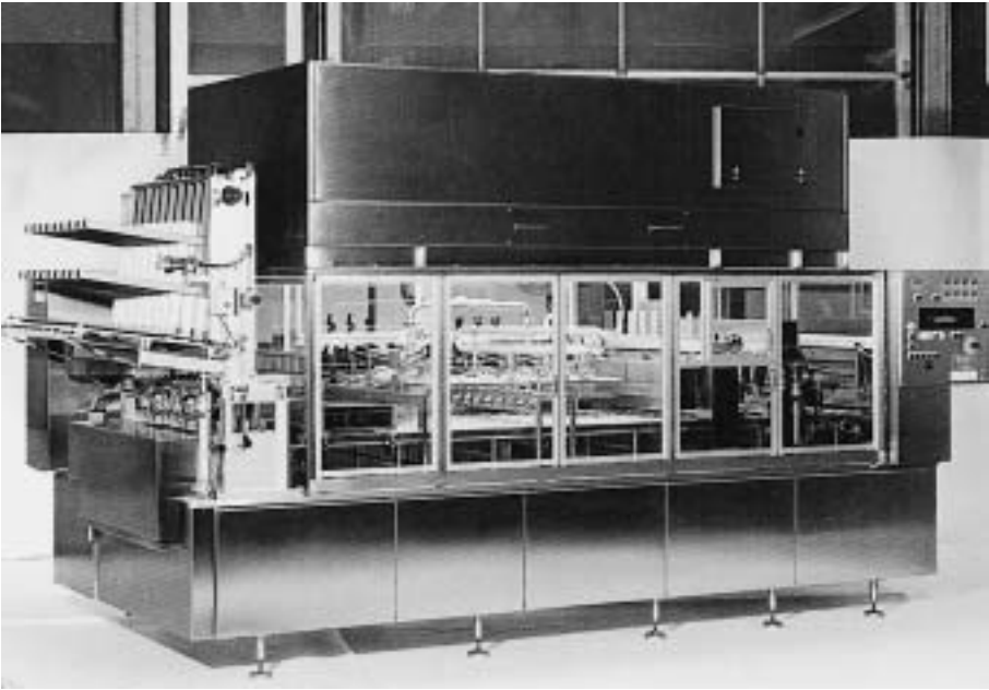
Fig. 3.60 An eight-lane Trepko cup filler
