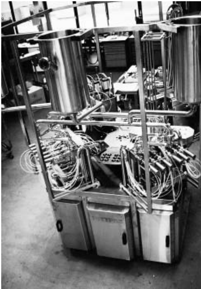
Fig. 3.59 View showing the rotary Hittpac AKH-051 series cup filler Note the two \times 6 cup pocket for multipack yoghurts. Reproduced by courtesy of Corporation Packaging, Farnham, U.K.
