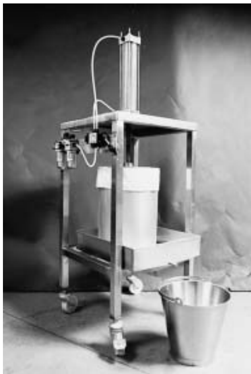
Fig. 5.14 Small-scale vertical press for the production of labneh anbaris or yoghurt cheese
