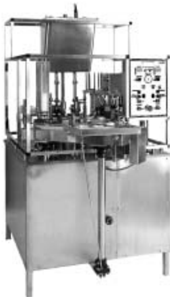
Fig. 3.12 Cockx rotary cup filler and sealer Reproduced by courtesy of C.K.X. Engineering, Sudbury, U.K.
