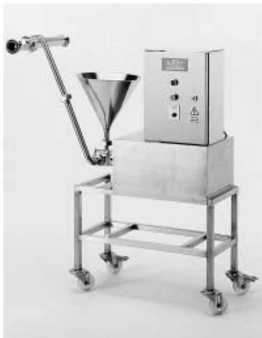
Fig. 3.53 View of the Clarendon fruit feeder/ripple pump with a static-in-line mixer Reproduced by courtesy of Clarendon Food & Dairy Equipment, Leaming Spa, U.K.
