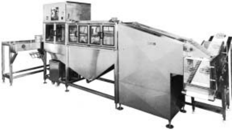
Fig. 3.51 View of an automatic can opening system
