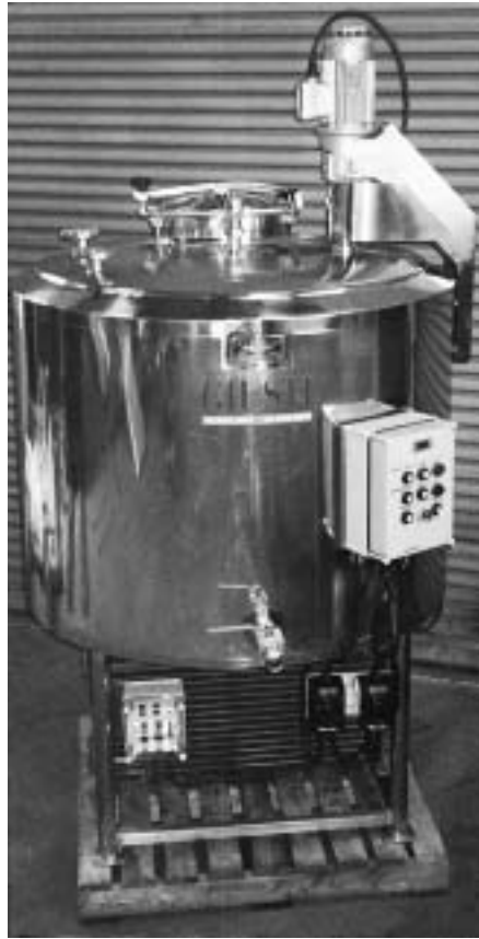
Fig. 3.6 Typical batch pasteuriser which can be used as a multipurpose vat for the production of yoghurt
