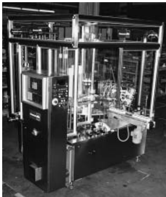
Fig. 3.10 Waldner Dosomat rotary-type yoghurt filling machine
