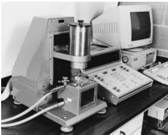
Fig. 10.7 Overall view of a rheometer linked to a computer to enable dynamic measurements of yoghurt structure to be made
