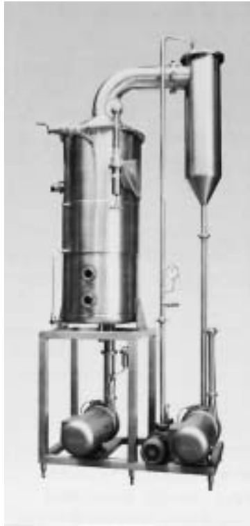
Fig. 3.17 View of an internal evaporation and de-aeration plant used on a yoghurt processing line
