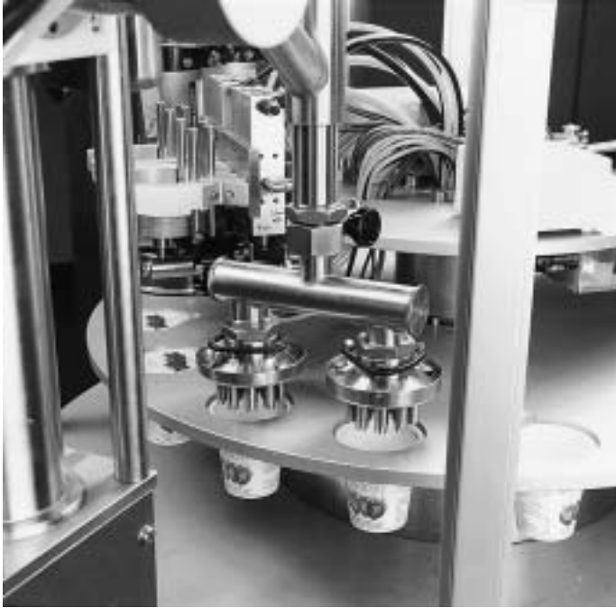
Fig. 3.11 Filling heads on Turbo Rotafil packaging machine Reproduced by courtesy of GEI International, Woburn Sands, U.K.
