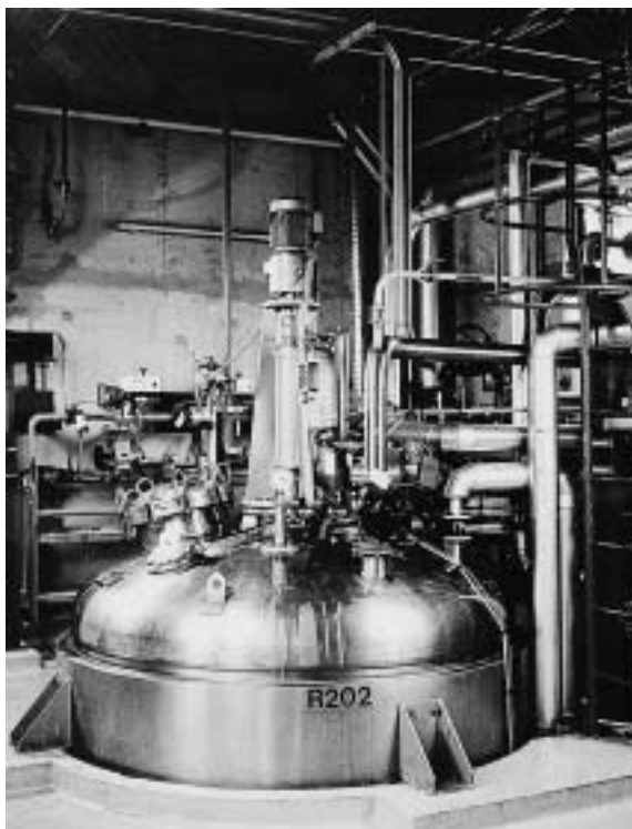
Fig. 8.4 Fermentor for the production of starter culture concentrate prior to freeze drying
