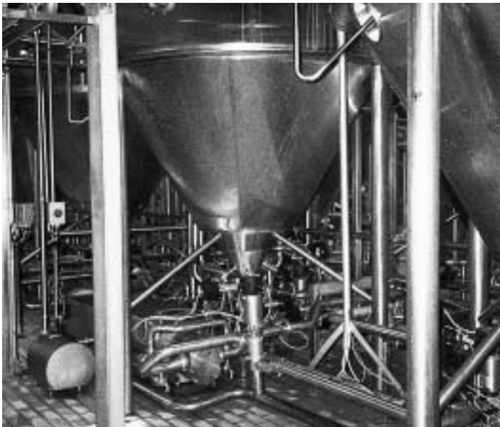
Fig. 3.37 Conical-shaped fermentation tank designed for easy discharge of yoghurt from the base
