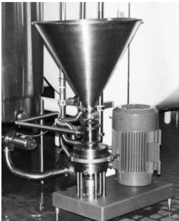
Fig. 3.20 Tri-Clovers dual-stage Tri-Blender® Reproduced by courtesy of Tri-Clover Inc., Kenosha, U.S.A.
