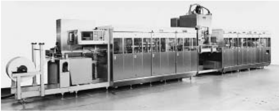
Fig. 3.63 The Illig FS 51 aseptic filling machines
